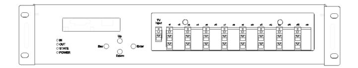
Outline the menu of High Power Optical Amplifier. For the description of all instructions, please refer to the panel shown below. Through the buttons on the right side of the LCD screen, you can scroll through all the menus of the large light.
